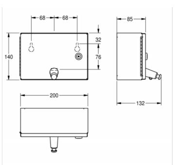
Soap dispenser for wall mounting, stainless steel, surface satin finished, material thickness 0.8 mm, folded front cover, cylinder lock with Franke standard key, suitable for liquid soaps and lotions, 1 liter soap tank, push button on front, incl. stainless steel screws and dowels.
