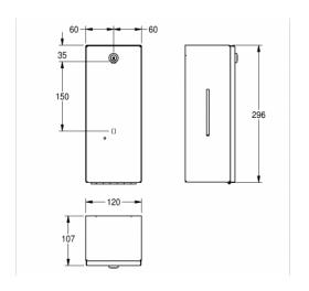
Touch free soap dispenser for wall mounting, stainless steel, surface satin finished, material thickness 20 gauge folded front cover, cylinder lock with Franke standard key, infrared sensor activity for non-touch operation, LED-light shows battery status, needs 4 pcs. 1.5 V (=9 V) Alkaline AA batteries, suitable for liquid soaps and lotions, 800 ml soap tank, depending on soap between 0.6 and 1.1 ml is dispensed, incl. stainless steel screws and dowels.
