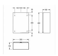
Waste bin for wall mounting, stainless steel, surface satin finished, material thickness 0.8 mm, rounded edges, mounting either with mounting bracket or directly onto the wall, incl. stainless steel screws and dowels.
