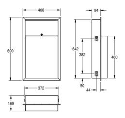
Waste bin for recessed mounting, stainless steel, surface satin finished, material thickness 0.8 mm, rounded edges, cylinder lock with Franke standard key, mounting with in-wall frame, incl. stainless steel screws and dowels.
